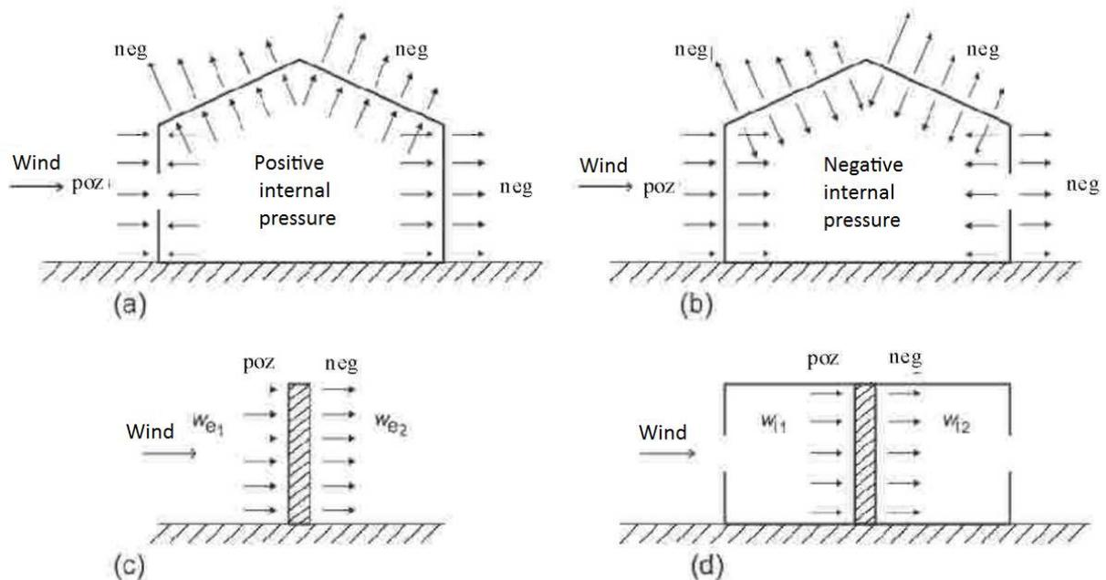
**Fig.1.** Representation of the pressure / suction on surfaces in the Code CR-1-1-4 / 2012
