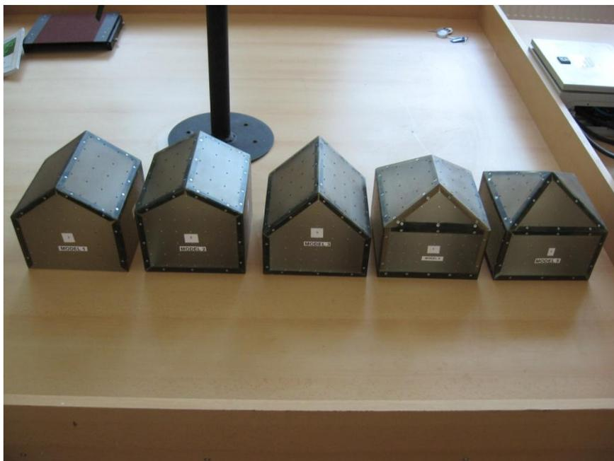
**Fig. 5.** *The greenhouses models developed for experimental research*
