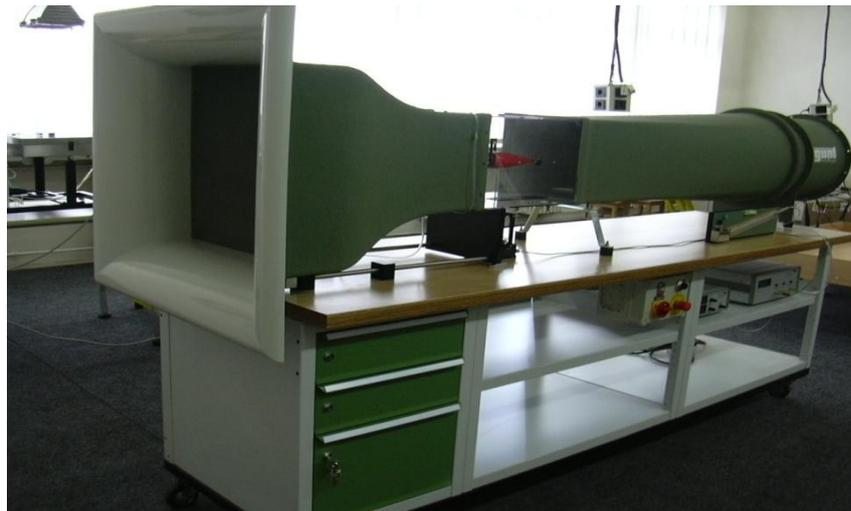
**Fig. 6.** HM 170 Aerodynamic Educational Wind Tunnel G.U.N.T. Gerätebau GmbH, Barsbüttel, Germany [11], [8]
