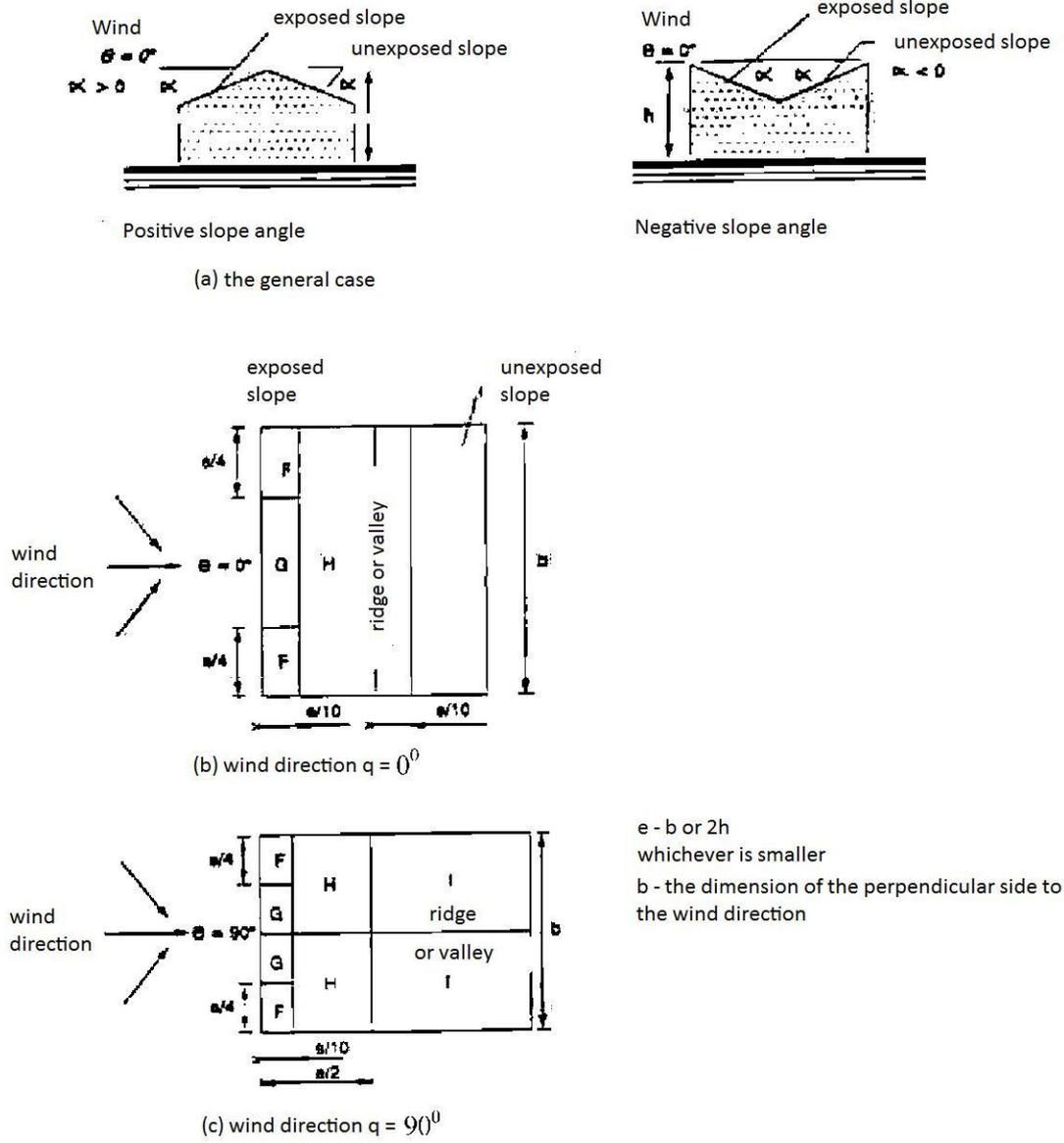
Fig. 2. Notation for roofs with two slopes of the Code CR-1-1-4 / 2012
