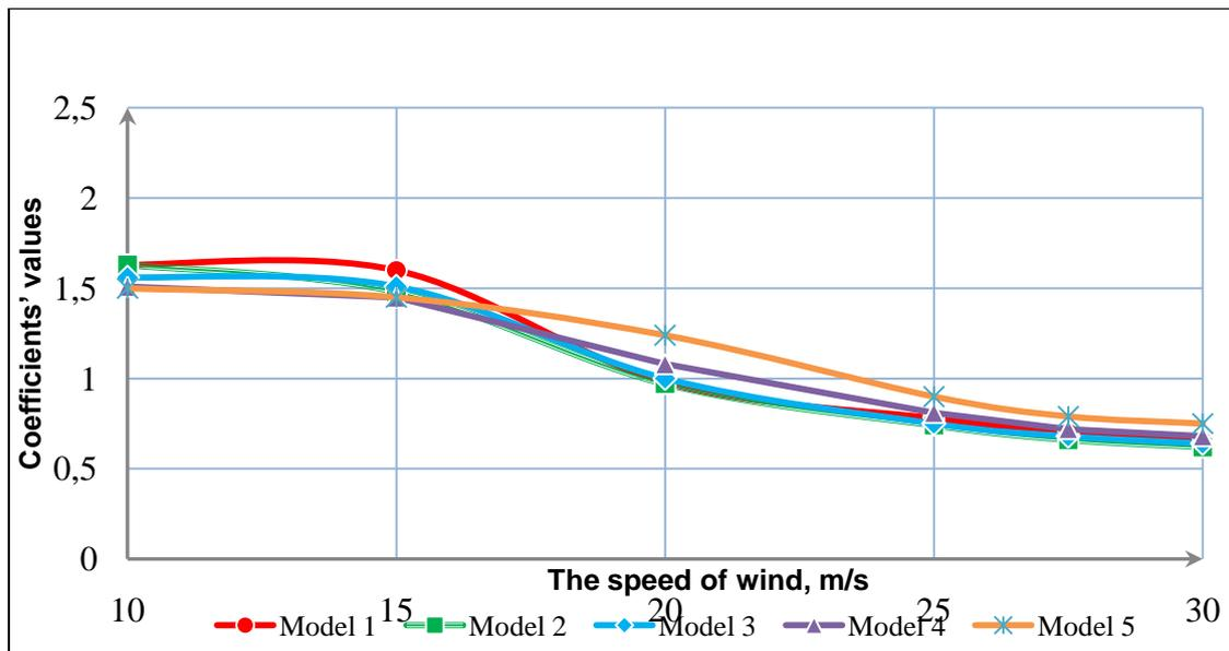
Fig.8. The variation of aerodynamic drag coefficient of the models by lateral airflow action
