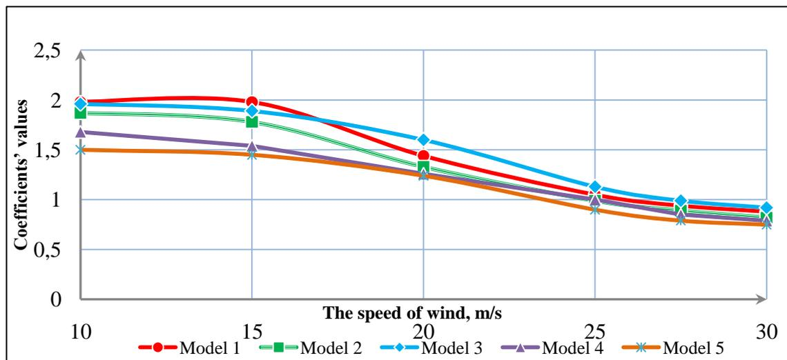
Fig. 7. The variation of aerodynamic drag coefficient of the models by frontal airflow action
