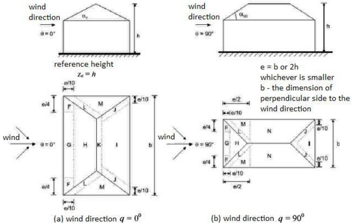
Fig.3. Notation for roofs with four slopes of the Code CR-1-1-4 / 2012 Wind direction
