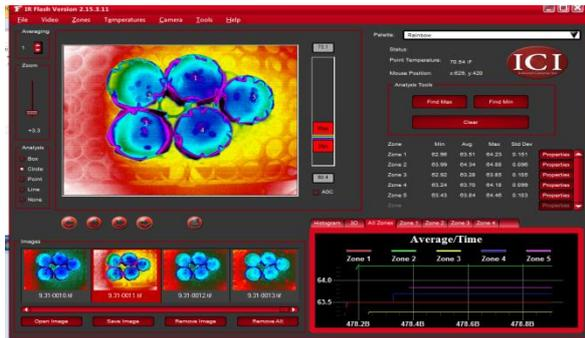
Fig. 2. Thermal image of the seed swelling process.
